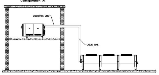
\* Liquid line riser should not exceed 15 feet from base of air-cooled condenser.
